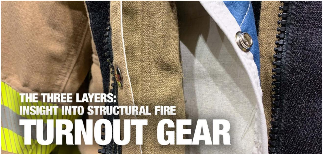
Effective structural fire turnout gear not only protects first responders from flames, it also prevents heat, liquids, chemicals, and potentially toxic substances—such as carcinogens—from harming a firefighter. Each layer of turnout gear—outer shell, moisture barrier, and thermal liner—utilizes highly technical fabric technology to create a system that works together to provide multi-hazard protection. We explore how each layer plays its part in protecting firefighters as they respond to calls.
